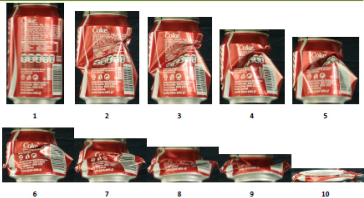
Figure 7 FEM analysis progressive views of aluminium can axial collapse
