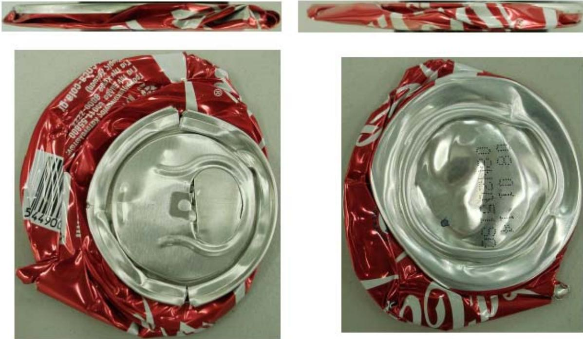
**Figure 6** Experimental terminal views of aluminium can axial collapse: side views (top figures), top view (bottom left) and bottom view (bottom right)
