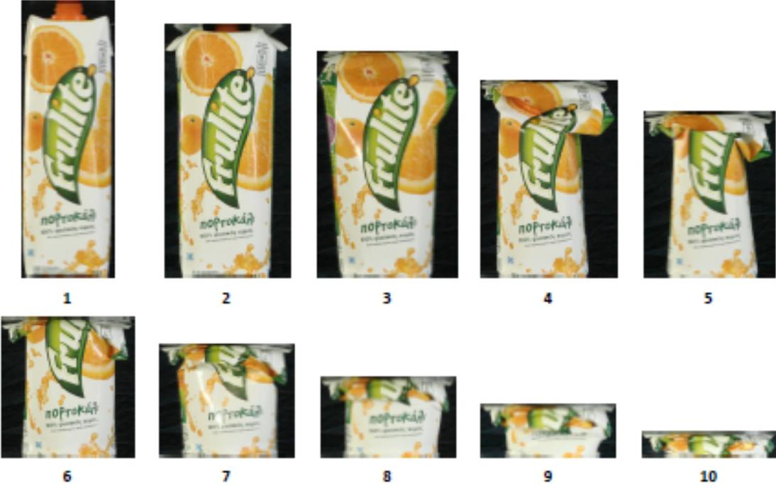
Figure 13 FEM Analysis and experimental progressive views of drink cardboard box axial collapse
