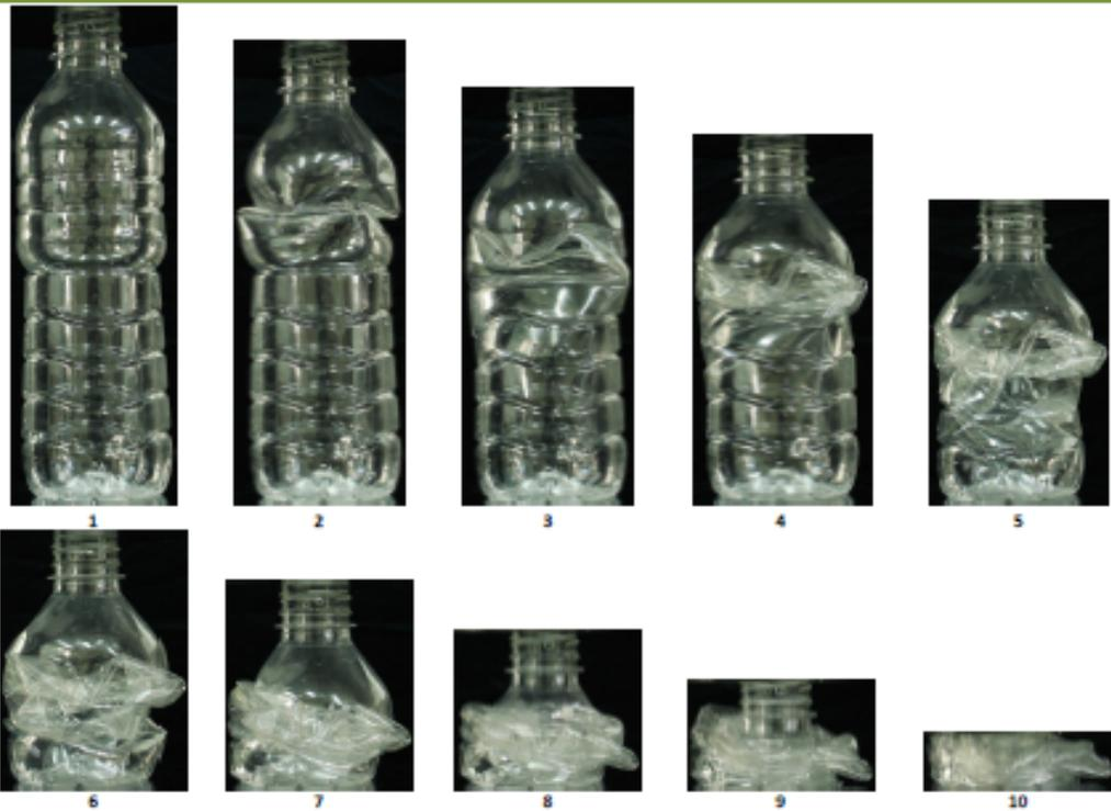
**Figure 11** FEM Analysis and experimental progressive views of PET bottle axial collapse
