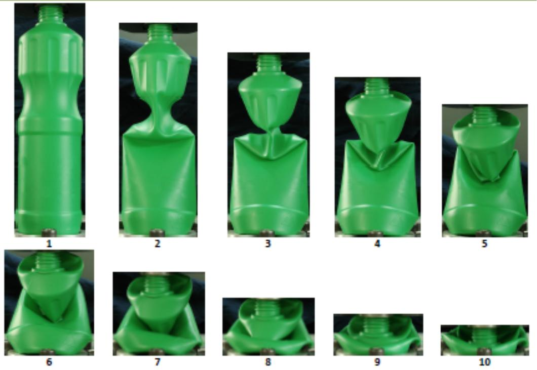
Figure 9 FEM Analysis and Experimental progressive views of HDPE bottle axial collapse
