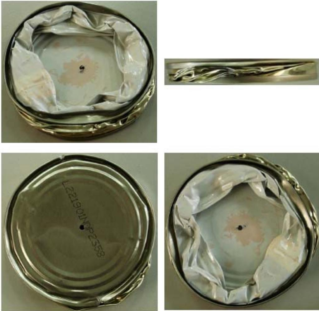
**Figure 4:** Experimental terminal views of tin-plate can axial collapse: isometric view (upper left), side view (upper right), bottom view (bottom left) and top view (bottom right)
