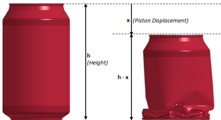
**Figure 14: Compression ratio and piston displacement, example of aluminium can**
