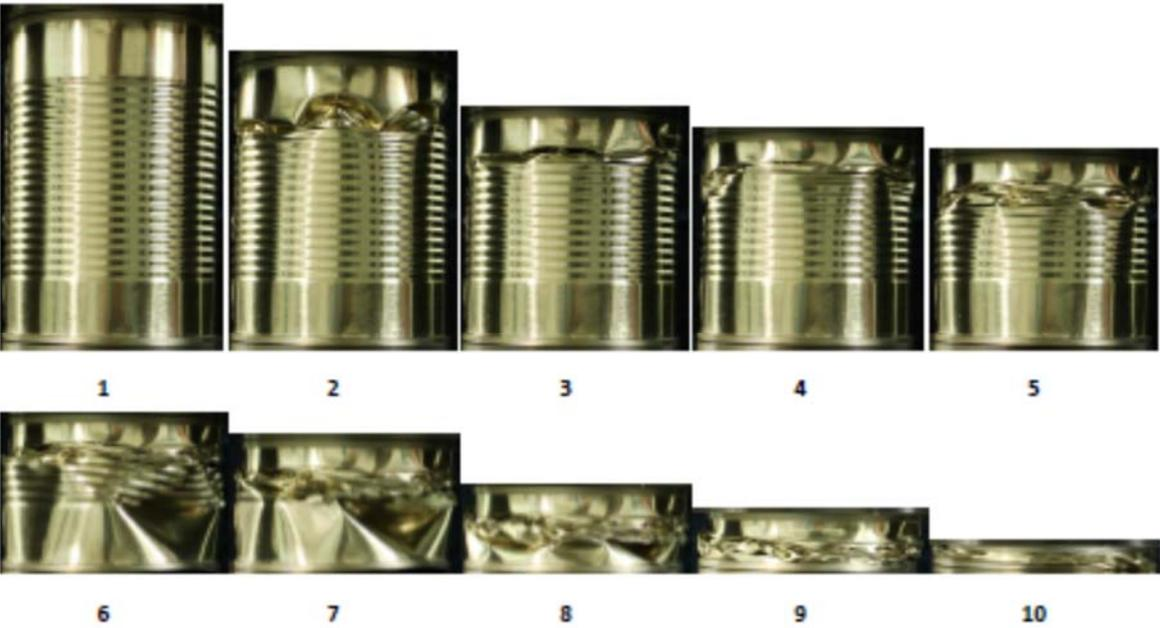
Figure 5: FEM analysis and experimental progressive views of tin-plate can axial collapse
