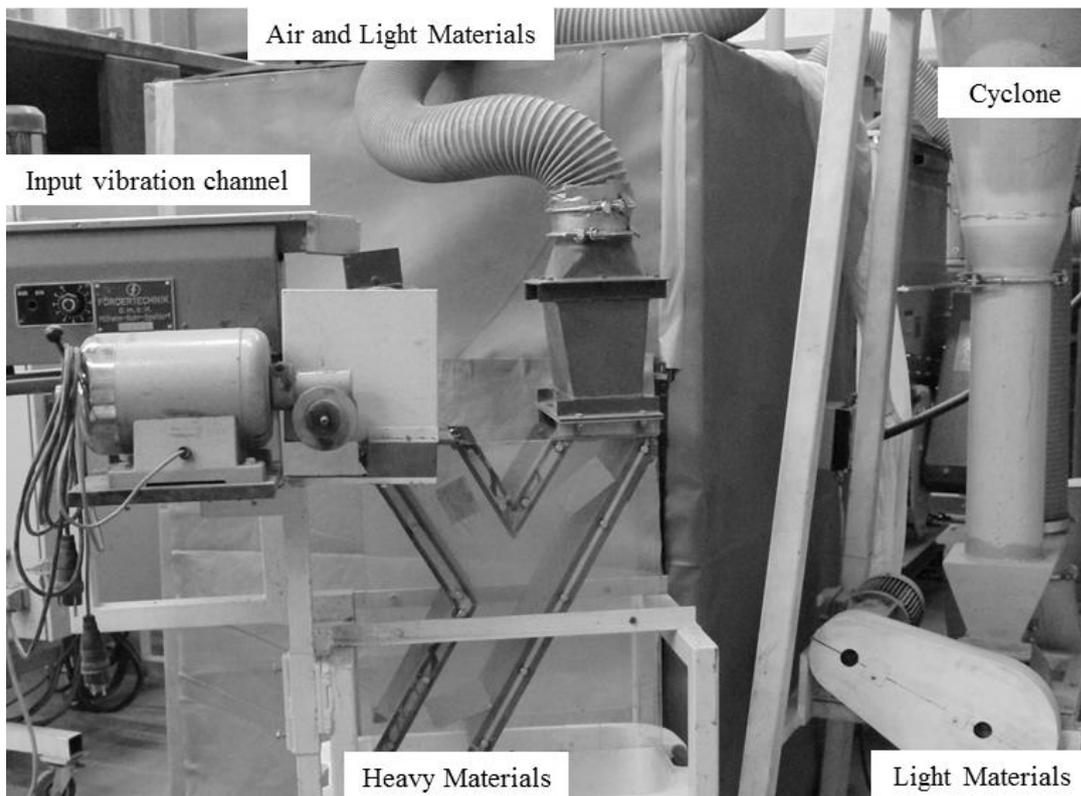
**Figure 5:** Zick-Zack Air sifter in the technical lab of I.A.R. Aachen.
