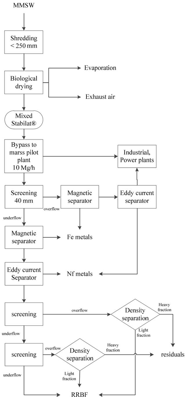
**Figure 8:** Process flow chart of MARSS demo plant
