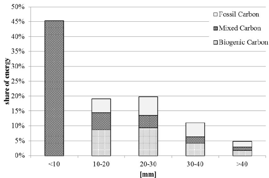
**Figure 3:** Distribution of the net energy content across the particle size fractions including the allocation of the origin of the energy to fuel groups. (Clausen et al., 2013)
