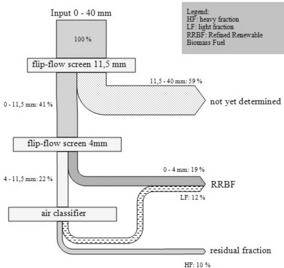
**Figure 7:** Sankey Diagram showing the mass proportions for sieving and wind sifting.
