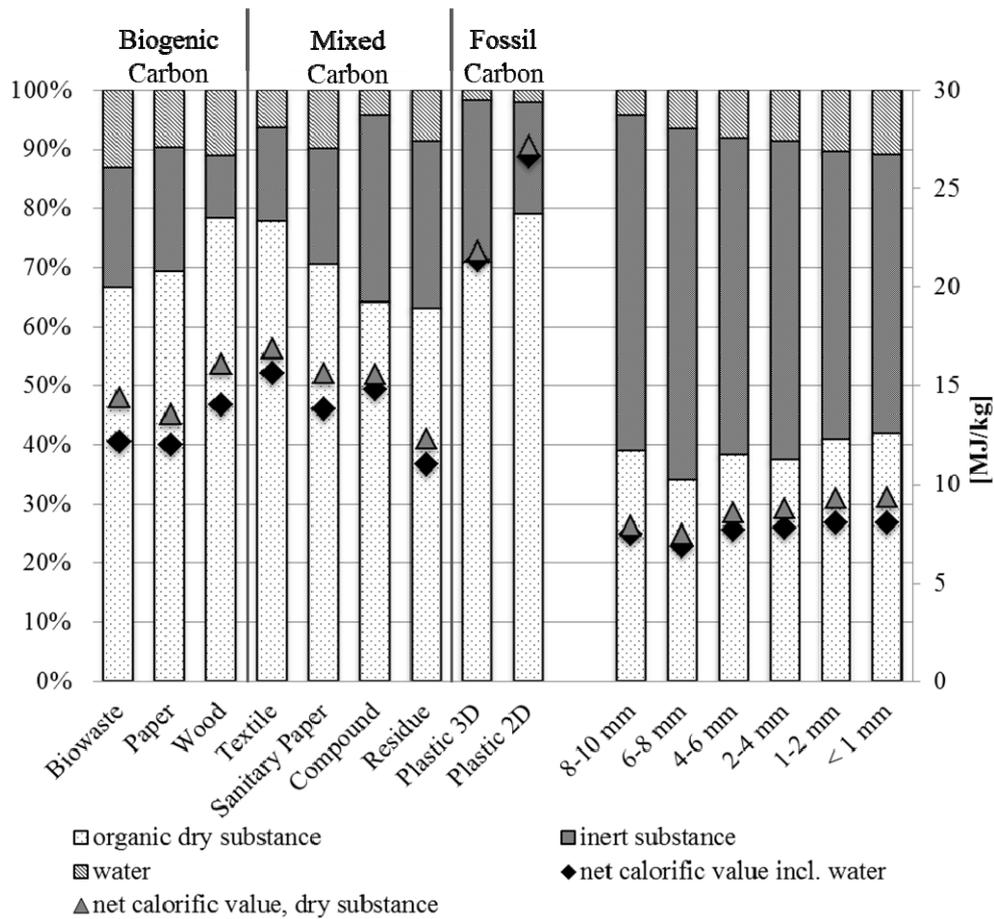
**Figure 2:** Relative composition of the material fractions in terms of water, organic dry substance and inert substance (primary y-axis) combined with the specific net calorific value (d and ar) (secondary y-axis). (Clausen et al., 2013)
