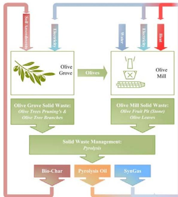
**Fig. 2** Waste management via Pyrolysis and the products utilization
