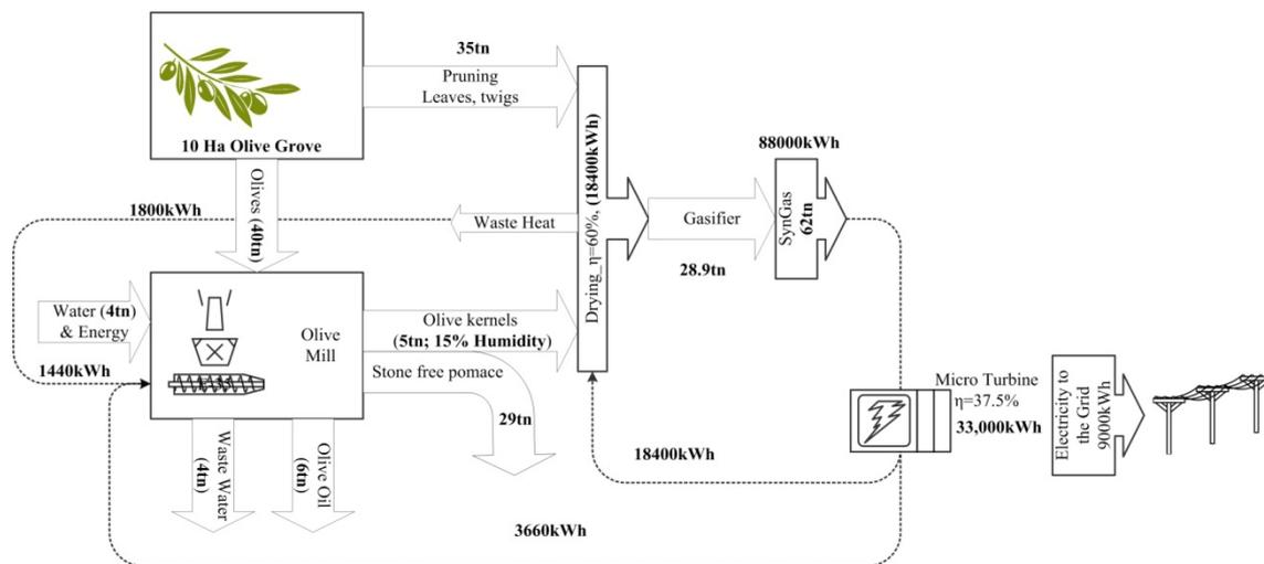
**Fig. 4** Energy and Mass balances (Gasification)
