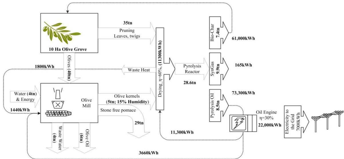
**Fig. 3** Energy and Mass balances (Pyrolysis)
