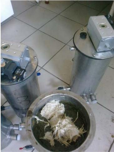
**Figure 1.** Batch anaerobic digestion with pre-treated chicken feather
