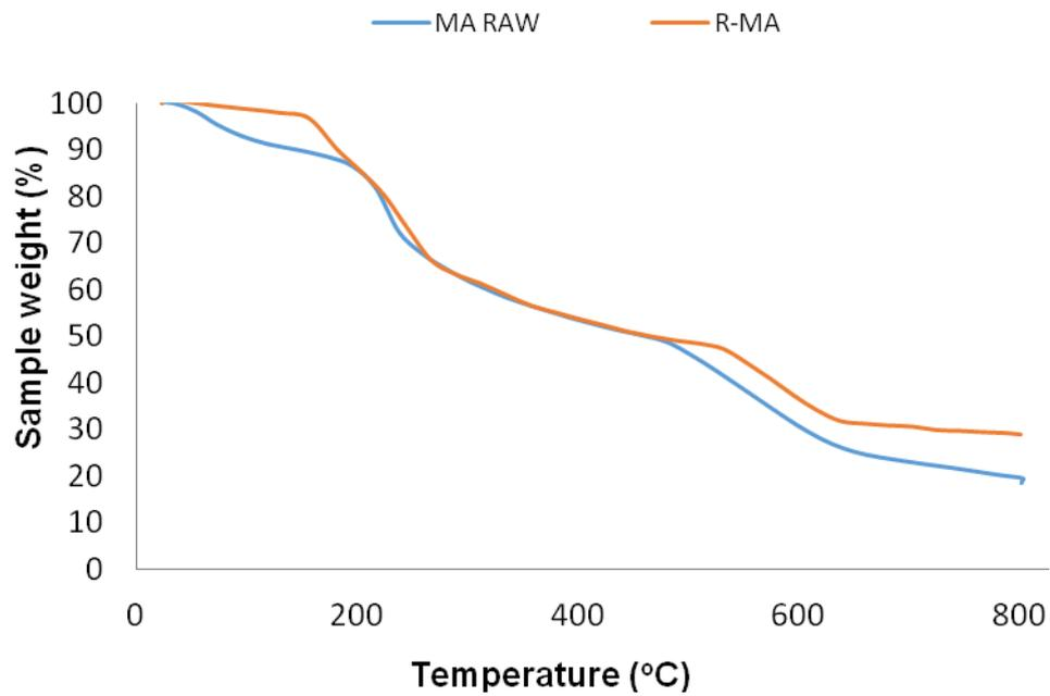
**Fig. 1** TG pyrolysis profiles of *Gracilaria gracilis* residue after phycolibiprotein extraction (R-MA) and raw *Gracilaria gracilis* at a heating rate of 10°C/min (nitrogen atmosphere).
