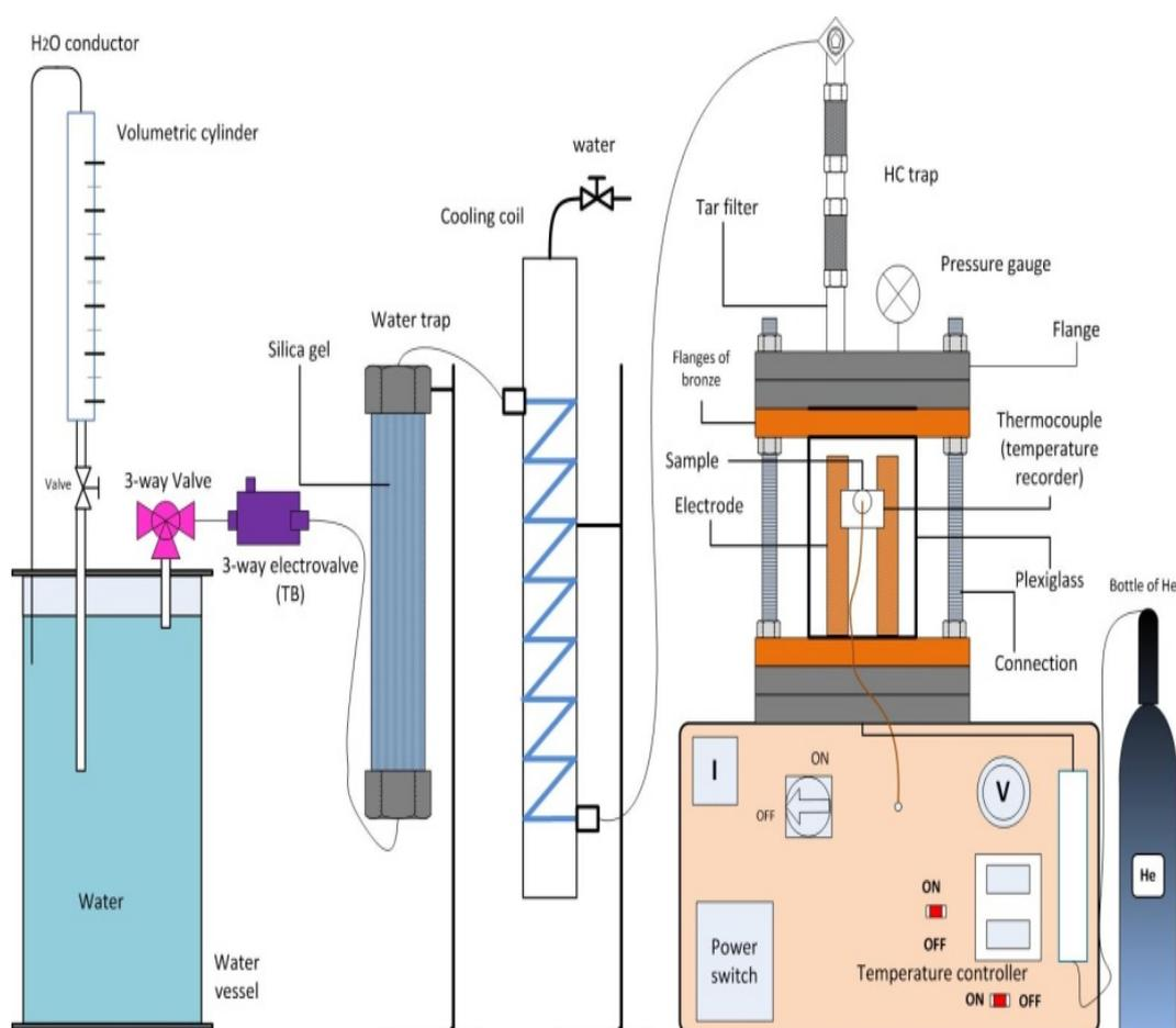
**Figure 1** Experimental set up for fast pyrolysis. .
