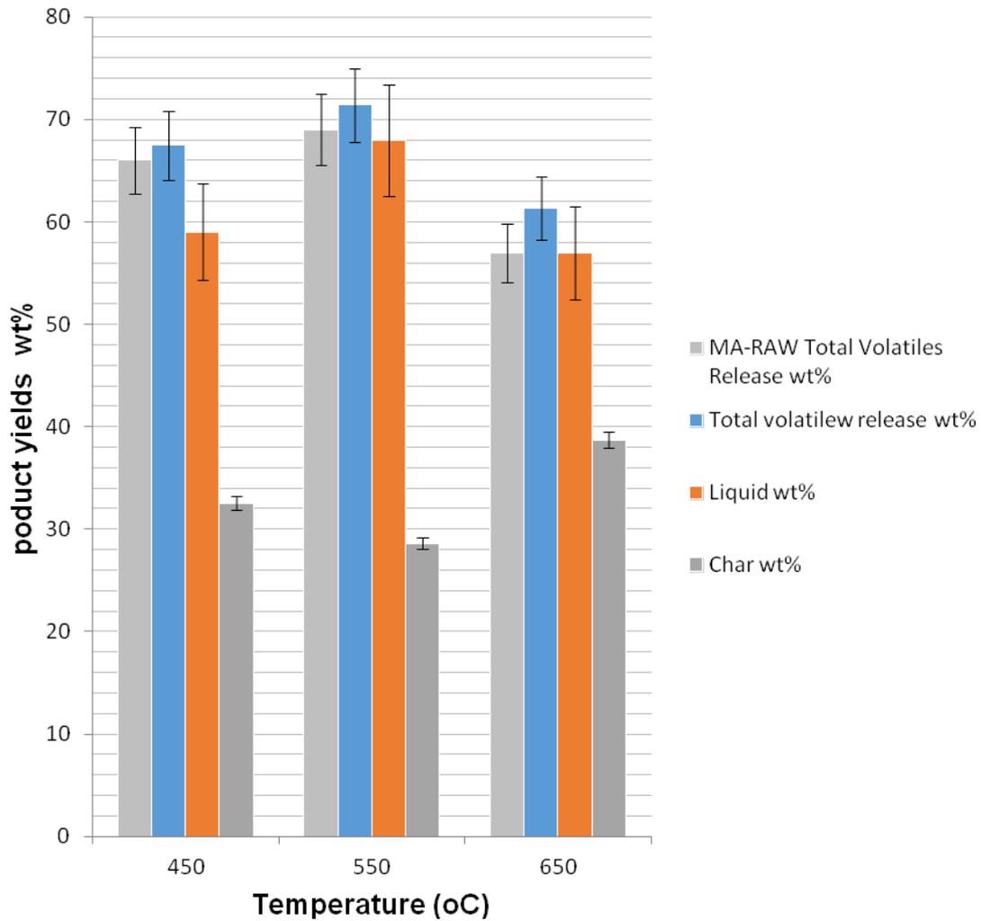
**Fig. 3** Total volatiles release of macroalgae and the residue, as well as liquid and char yield results of the residue via fast pyrolysis at 450 °C, 550 °C and 650°C.
