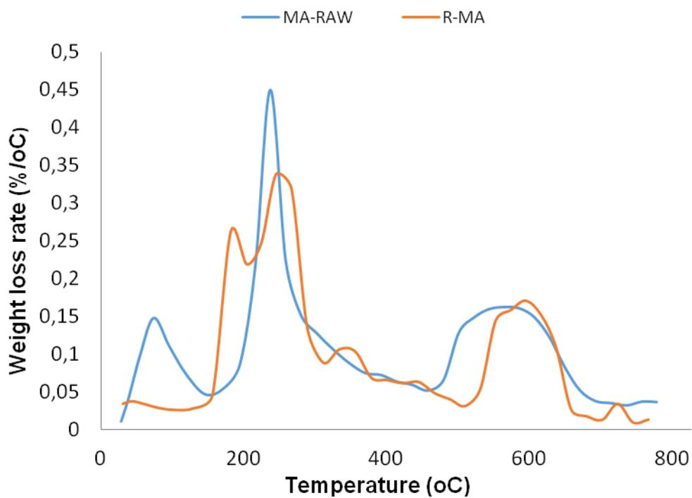
**Fig. 2** DTG curves of *Gracilaria gracilis* residue after phycolibiprotein extraction (R-MA) and raw *Gracilaria gracilis* at a heating rate of 10°C/min (nitrogen atmosphere).
