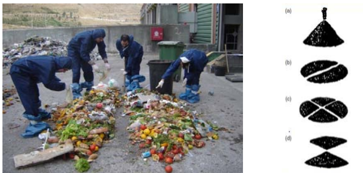
Figure 2: Coning and quartering procedure for selecting representative unprocessed waste samples
