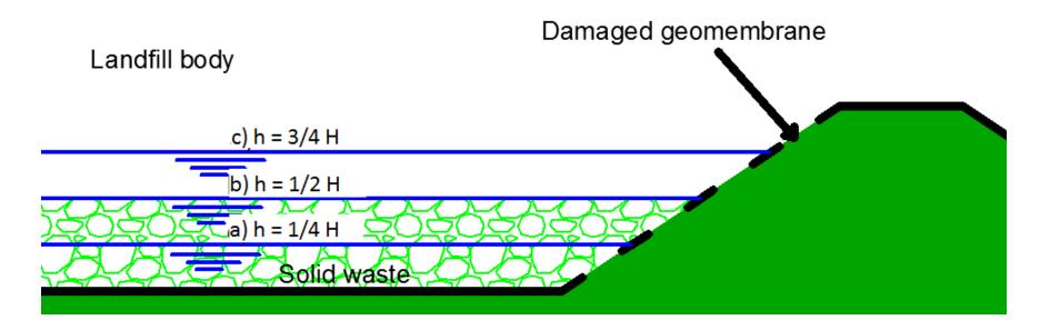
Outer slope toe of the wall is the critical area...
