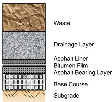
Figure 7: Example for an asphalt lining system
