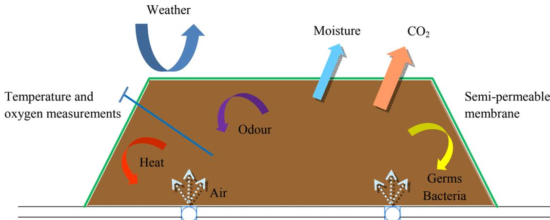
Figure 6: Heap cross section with membrane cover
