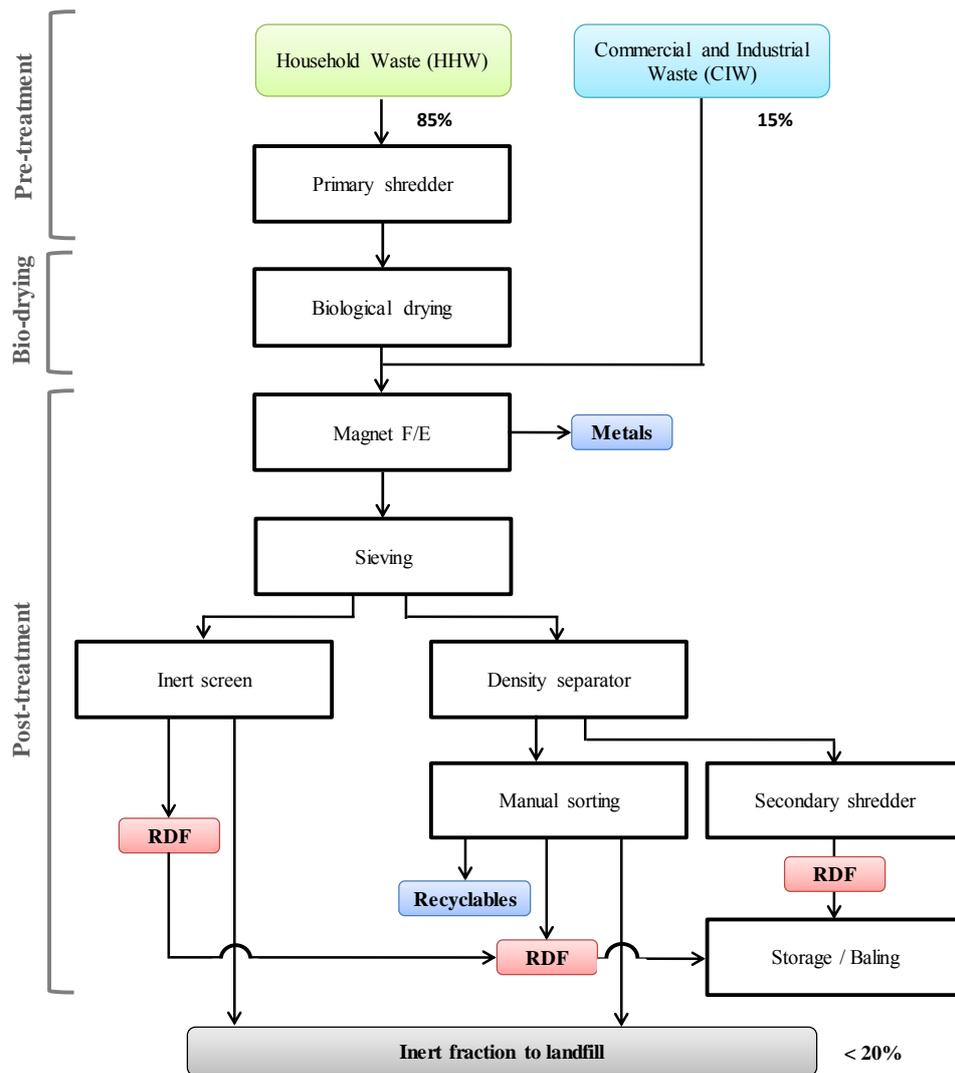
Figure 5: Flow chart of MBT process
