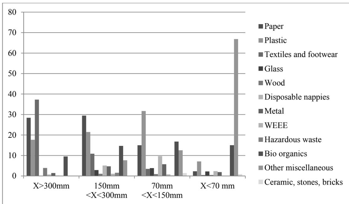
Fig. 4: Content of municipal waste fractions sorted by sieves with meshes 300 mm, 150 mm, 70 mm
