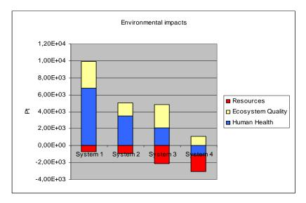
Figure 5: Total Environmental Impacts for each one of the four systems. The bars represent the average value of the sensitivity analysis scenarios of each system. (Method eco-indicator 99, total weighted results, single score)
